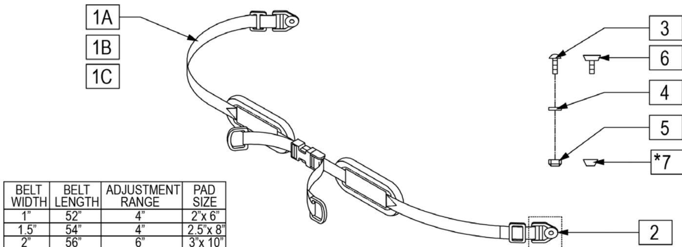
NOTE : ITEM 7 CHANNEL NUT IS USED WHEN ORDERING IN CONJUNCTION WITH CUSTOM CONVENTIONAL SEATING
