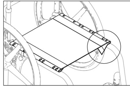
FOR PROPER FIT OPEN THE VELCRO FLAP ON THE UNDER SIDE OF THE SLING FOR INSTALLATION. THE SLING MAY MEASURE SHORT, BUT BY OPENING THE FLAP IT WILL ADJUST TO FIT THE FRAME.
