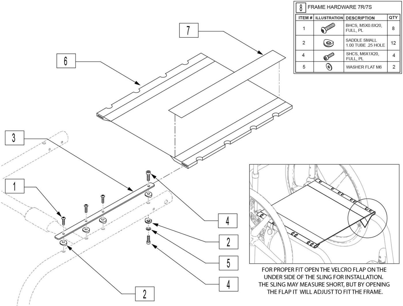
FOR PROPER FIT OPEN THE VELCRO FLAP ON THE UNDER SIDE OF THE SLING FOR INSTALLATION. THE SLING MAY MEASURE SHORT, BUT BY OPENING THE FLAP IT WILL ADJUST TO FIT THE FRAME.
