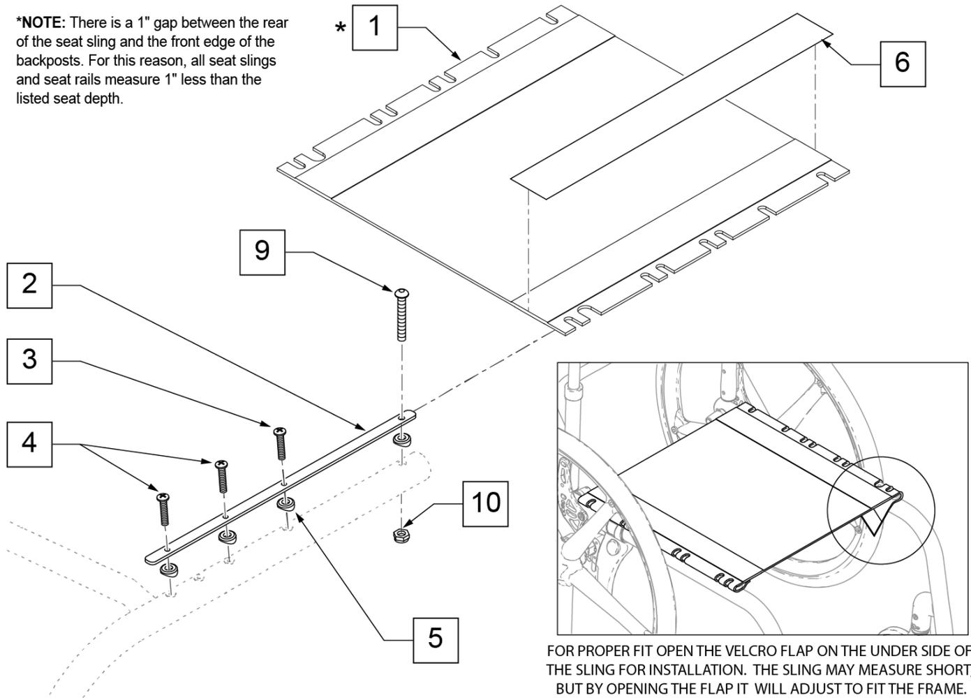
FOR PROPER FIT OPEN THE VELCRO FLAP ON THE UNDER SIDE OF THE SLING FOR INSTALLATION. THE SLING MAY MEASURE SHORT, BUT BY OPENING THE FLAP IT WILL ADJUST TO FIT THE FRAME.
