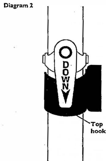
**NOTE:** The back is properly secured when the bottom pins are resting in the lower post brackets and the upper quick release quarter turn brackets are installed above the back support's top hook brackets with the quick release mechanism pointing down.
