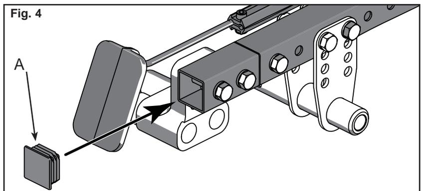
1. (Fig 1) Remove base frame end plug (item A) from right base frame tube. Remove the Pedal Assembly (item M) by unscrewing the two hex head screws (item F). Set screws and washers (item G) aside for reinstallation.
