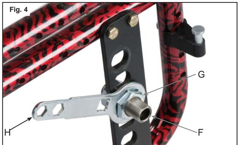
9. Once loosened turn both the inside (I) and outside (G) axle nuts clockwise until the Axle Sleeve protrudes 1" from the outside axle nut. (Fig 5). Tighten the axle nuts securely.
