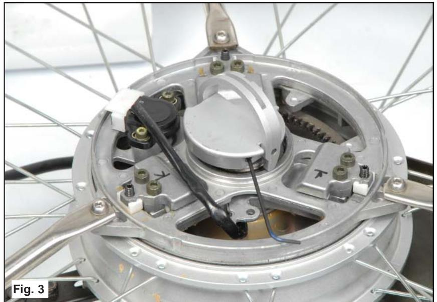
3) Hold the flat spots on the axle with an 8mm Wrench, while turning the Plate Assembly counter clockwise. This will remove the Plate Assembly from the axle.
