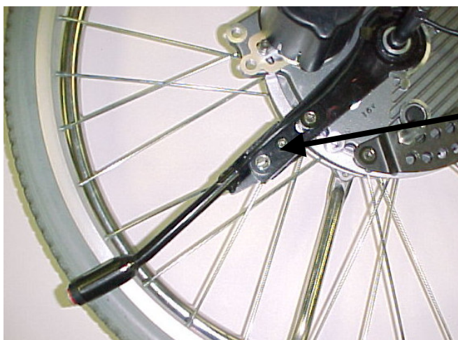
Figure 4: On/Off Switch w/o 45° Bracket
