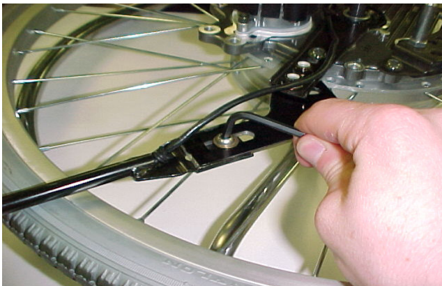
Figure 8: Attachment of On/Off Bracket
