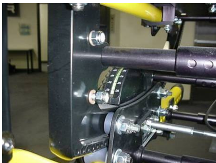
Figure 10: Attaching a 1/4-28 Nylock Nut
