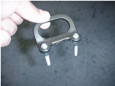
Figure 7: Bolt and washer sets placed on front bracket
