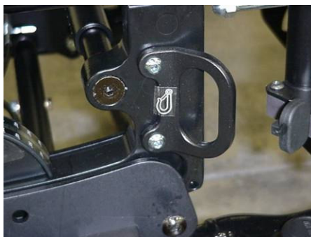
Figure 8: Orientation of front bracket relative to wheelchair
