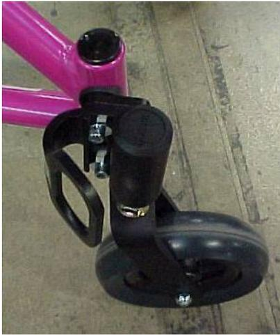
**Figure 12:** Final Setup with Caster Barrel Leading
