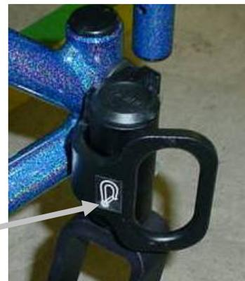
**Figure 11:** Transit Mount Location Decal Placement
