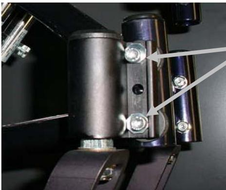
Remember Orientation of Eccentric Washer to help in the reinstallation in later steps.
