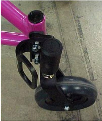
**Figure 12:** Final Setup with Caster Barrel Leading
