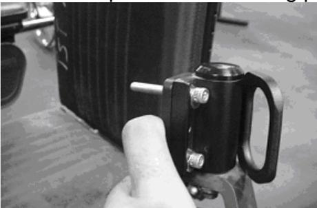
**Figure 9:** Bracket attached to wheel mount
