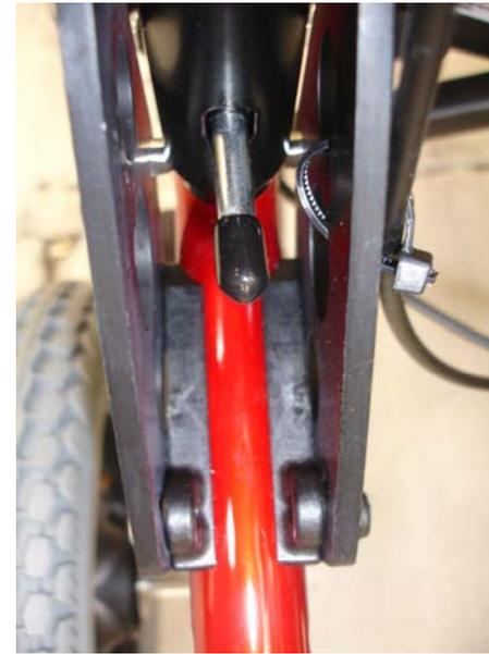
**Figure 1a:** New Saddles and Vertical Supports
