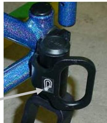
**Figure 11:** Transit Mount Location Decal Placement
